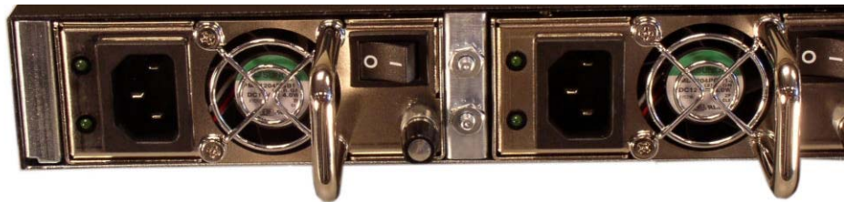
Figure 6 - 103. Power Supply A and B Installed
