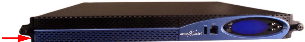
Figure 6 - 104. Removing the Front Bezel
