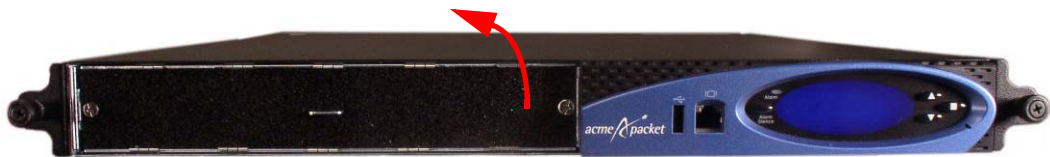
Figure 6 - 105. Removing Air Filter from Chassis
