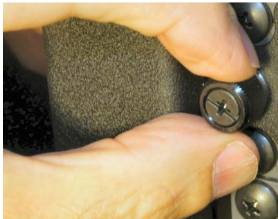
Figure 2 - 14. Securing the Chassis to the Rack
