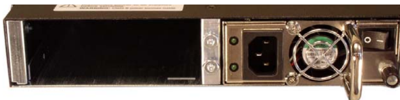
Figure 6 - 99. Power Supply Removed
