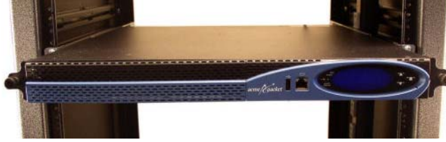
Figure 4 - 61. Installing the Chassis into the Equipment Rack
