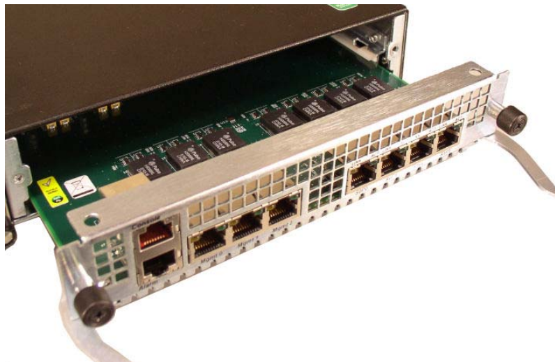
Figure 6 - 116. Removing the NIU
