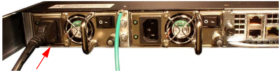
Figure 4 - 69. Connecting the Power Cord to Power Supply B
