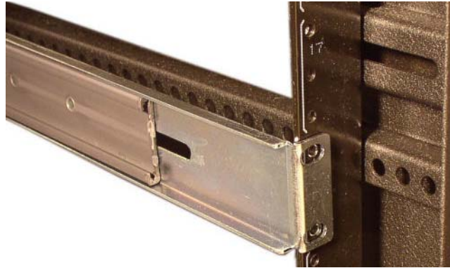
Figure 4 - 48. Aligning the Stationary Rail with the Equipment Rack
