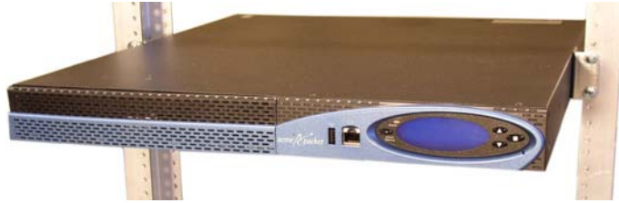
Figure 4 - 65. Acme Packet 4500 Center-Mounted in a Two-Post Equipment Rack
