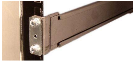
Figure 4 - 54. Stationary Slide Securely Attached to the Equipment Rack
