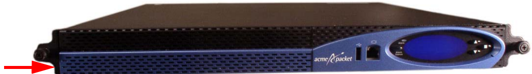
Figure 6 - 113. Re-Installing the Fan Bezel
