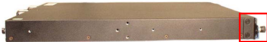
Figure 4 - 57. Chassis Ear Secured to the Chassis
