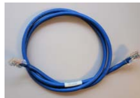
Figure 6 - 127. Cat 5/6 Ethernet Cable
