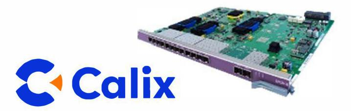
The Calix E7-2 GPON-8 line card provides eight ITU G.984-compliant Gigabit Passive Optical Network (GPON) interfaces and four Gigabit Ethernet (GE) interfaces, along with two ports of integrated 10-Gigabit Ethernet. The E7-2 GPON-8 line card can be plugged into one or both of the two universal slots within a Calix E7-2 shelf.
